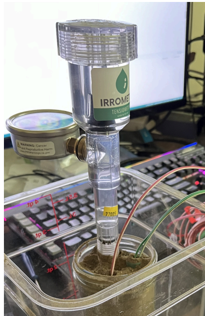
Figure 17: The calibrated sensor and our sensors in the soil for testing
